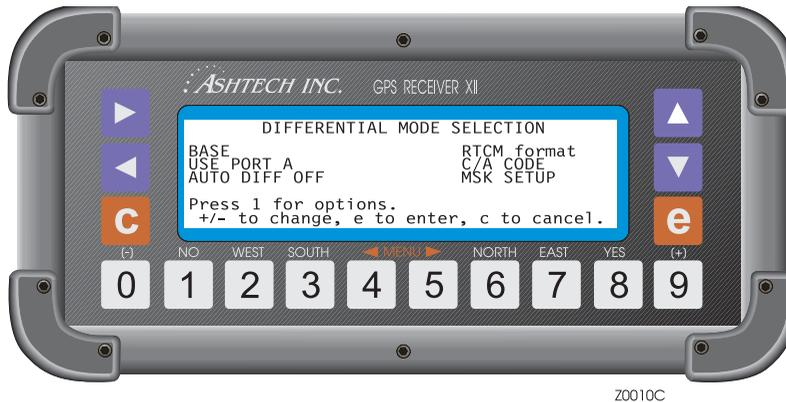
**Figure 2.7.** Differential Mode Selection Screen
