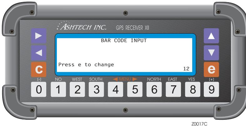
**Figure 3.47.** Screen 12 - Bar Code Control
