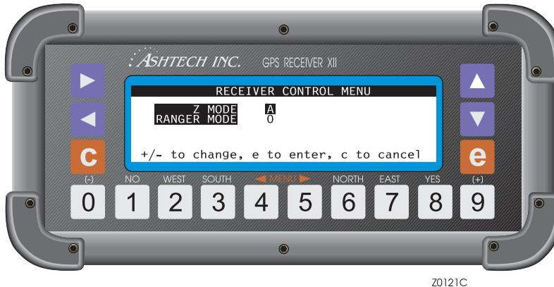
Figure 3.11. Receiver Control Subscreen
