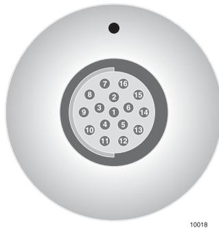
**Figure 1.5.** RS232 Connector (Port 1, Port 2)
